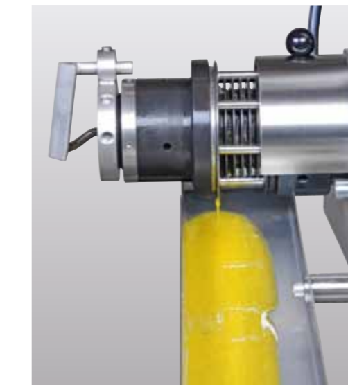
Pressing Cylinder with optimised oil outlet
